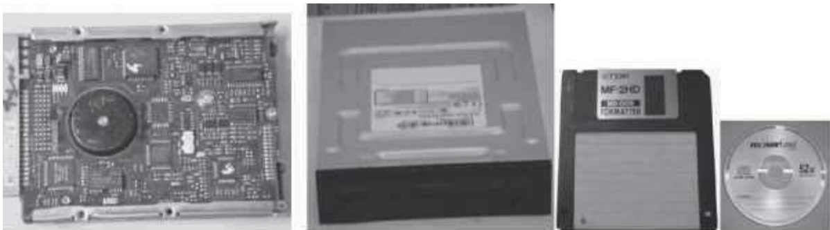
Figure 1.13 Storage devices (i) Hard disk drive, (ii) DVD drive, (iii) Floppy disk, (iv) CD
